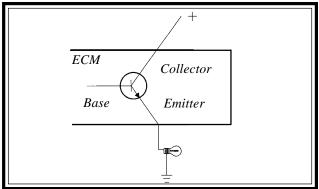
When voltage is supplied to the base the light turns on.
