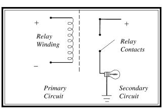
When voltage is applied to the relay winding the light turns on.
