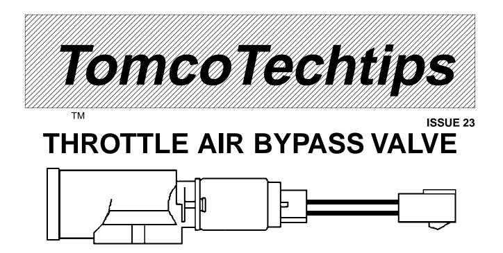
Ford uses an idle air bypass valve, sometimes called a throttle air bypass valve (TABP), to control the idle on its multipoint injection systems. The TABP is located on the throttle body or on the air induction system before the throttle body.
