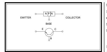
material sandwiched between two N type materials. The P material or region in this case is called the base. The two outer N regions are called the emitter and collector. As in the PNP transistor the base region is thinner and is lightly doped relative to the emitter and collector. An example of a NPN
