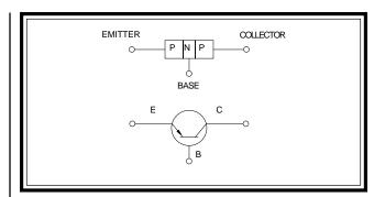
The bipolar junction transistor (BJT) is closely related to the PN junction diode we have just studied. The BJT is also made from the semiconductor materials of germanium and silicon. But instead of just two semiconductive materials joined together, the BJT has three semiconductive materials joined. This means there is a possibility of two different types of semiconductor arrangements, a PNP or a NPN arrangement.
