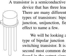
device that has three leads. There are many different types of transistors: bipolar junction, unijunction, field effect to name a few.
